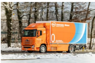
Caption: The hydrogen truck is designed to carry around 25 tons of goods and has a range of about 600 kilometers. (Source: Gebrüder Weiss / Stefan Peter)
