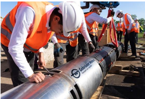
Capture: Groundhog Beta, the Innovation Award-winning tunnel drilling machine from Swissloop Tunneling (Source: Eugenio Valli)
